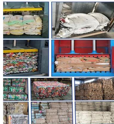
Vertical hydraulic baling machine is mainly suitable for compressing and packing of waste clothes, paper, cardboard, boxes, plastics, plastic bottles, cans, cotton, wool, yarn, textile products, woven bags, sacks, coconut shells, tires and other materials. The compressed bales are compact, firm and strong, which improves labor efficiency for customers, reduces storage space, facilitates packaging and transportation, and is conducive to environmental protection and waste recycling.
