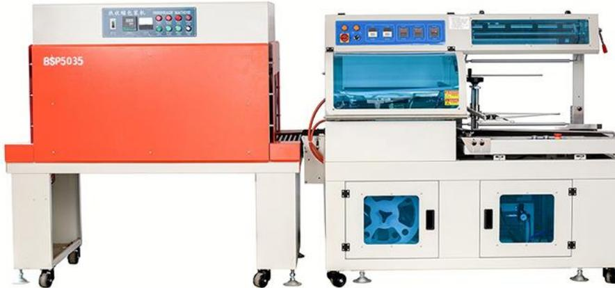
Automatic L sealing and shrinking machine adopts constant temperature heating technology and is used in conjunction with the shrinking furnace to make the temperature in the shrinking furnace reach a certain degree of heat and then heat the shrink film; when the product is wrapped, the sealing knife is used to perform the shrink film Heat sealing and cutting operation; then, put it into a thermostat for cooling treatment to make the product smooth and beautiful.
