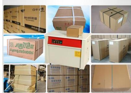
The semi automatic strapping machine uses a strap to bind the product or package, then tighten it and combine the two ends with a heating iron. The function of the strapping machine is to reinforce the packaged goods, so that the goods will not be scattered due to inadequate tying during handling and storage, and at the same time they should be tied neatly and beautifully.
