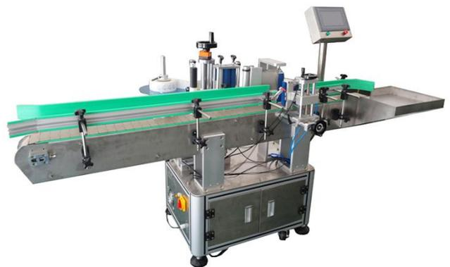
Round bottle labeling machine realizes labeling or filming on the circumferential surface of cylindrical and conical products, such as glass bottles, plastic bottles, etc. It can realize the functions of circumference, half circumference, circumference double-sided, circumference positioning labeling, etc., mainly including There are two ways of vertical labeling and horizontal labeling.
